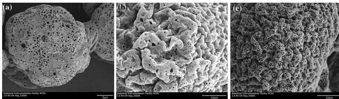
Fig. 1 SEM images of non-fibrous electrospun structures: a 0.8, b 3, and c 5 wt% PLA/DCM, scale bars = 5, 10, 10 μm, respectively
